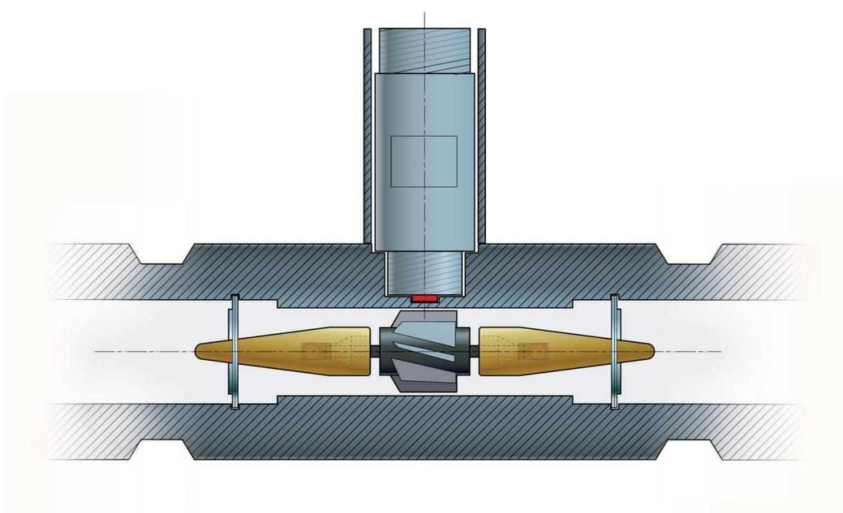
The Turbine flow meter (axial turbine) was invented by Reinhard Woltman and is an accurate and reliable flow meter for liquids and gases. It consists of a flow tube with end connections and a magnetic multi bladed free spinning rotor (impeller) mounted inside; in line with the flow. The rotor is supported by a shaft that rests on internally mounted supports.
